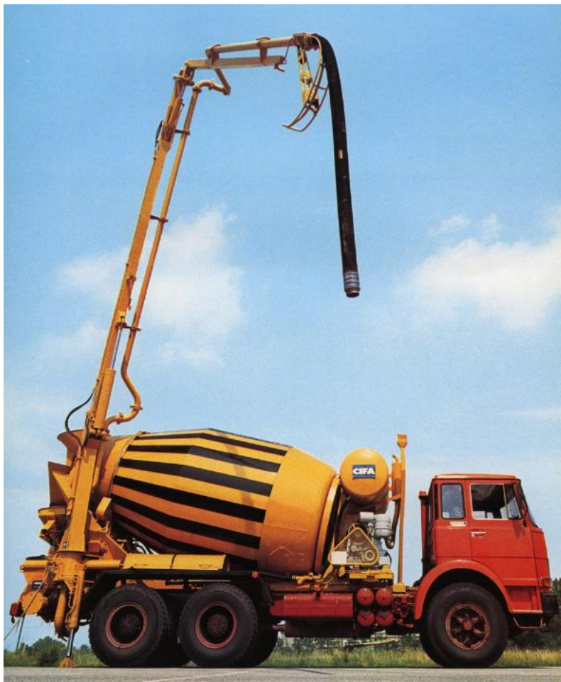
CIFA's first mixer-pump the 301B from 1974 was initially equipped with a 4 m 3 drum and 17 m two-section rear-mounted distributor boom.
